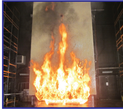
3 MW façade fire test on a large composite surface. Courtesy of RISE Safety/Fire Research
