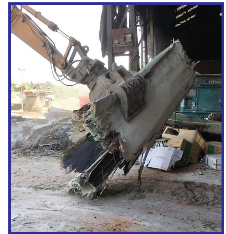
Wind turbine blade section ready for shredding and disposal in a cement kiln. Courtesy of Agecko
