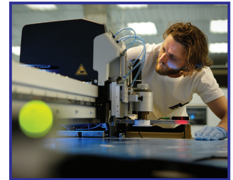
Kit cutting on a 12 metre ply cutter. Courtesy of A C Marine & Composites
