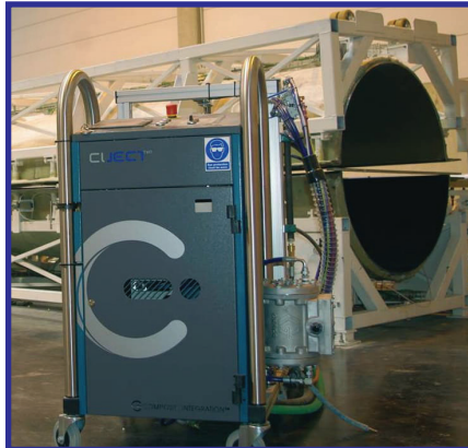
Composite Integration Ltd supplies resin injection equipment and processing technology for wind turbine blades. Courtesy of Composite Integration
