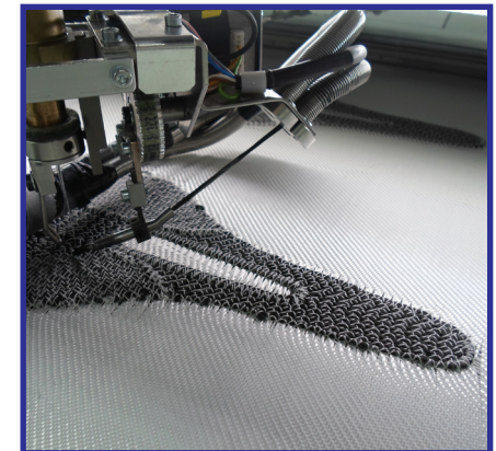
Shape Machining manufacture 2D and 3D preforms in carbon fibre, such as this bike seat, using an embroidery technique. Courtesy of Shape Machining
