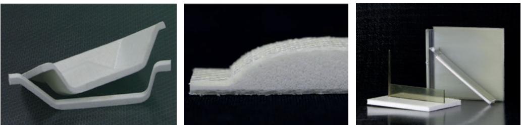
Fig. 3: Functionalized sandwich structures: thermoformed component (left), variable wall thickness (middle), co-injected structure (right)
