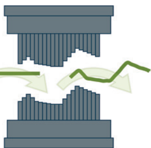
Fig. 1: Automated adjustment of the shape-adaptive tool geometry
