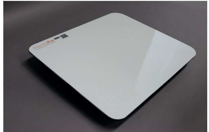
Fig. 4: Painted outer shell of the composite door structure
